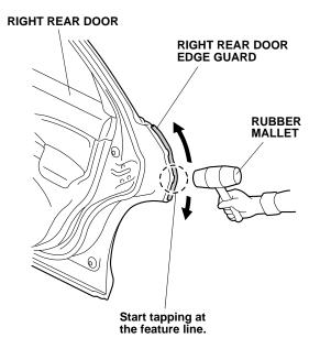
15. Repeat steps 3 through 14 to install the door edge guards on the left side of the vehicle.
