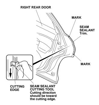
12. Apply touch-up paint to the cut seam sealant area, and let it dry thoroughly.
